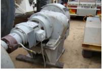
Westinghouse Multi-speed Motor with Reduction Drive and Wire Rope Winch 10 HP/1335 RPM/415 Volt - 14.5 Amps
